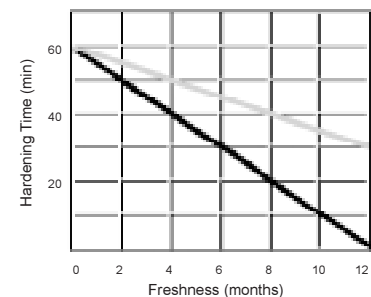
Figure 10. Hardening time for PFG-04 vs Storage Time. The black curve corresponds to a storage temperature of 18 °C and the grey curve to 4 °C.
